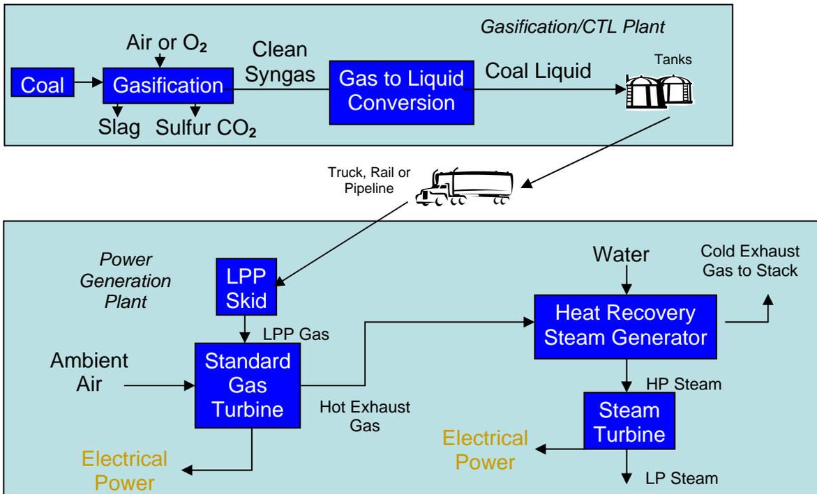
Figure 8: Scenario #3: Non-Integrated LPP Gas™ IGCC Plant
