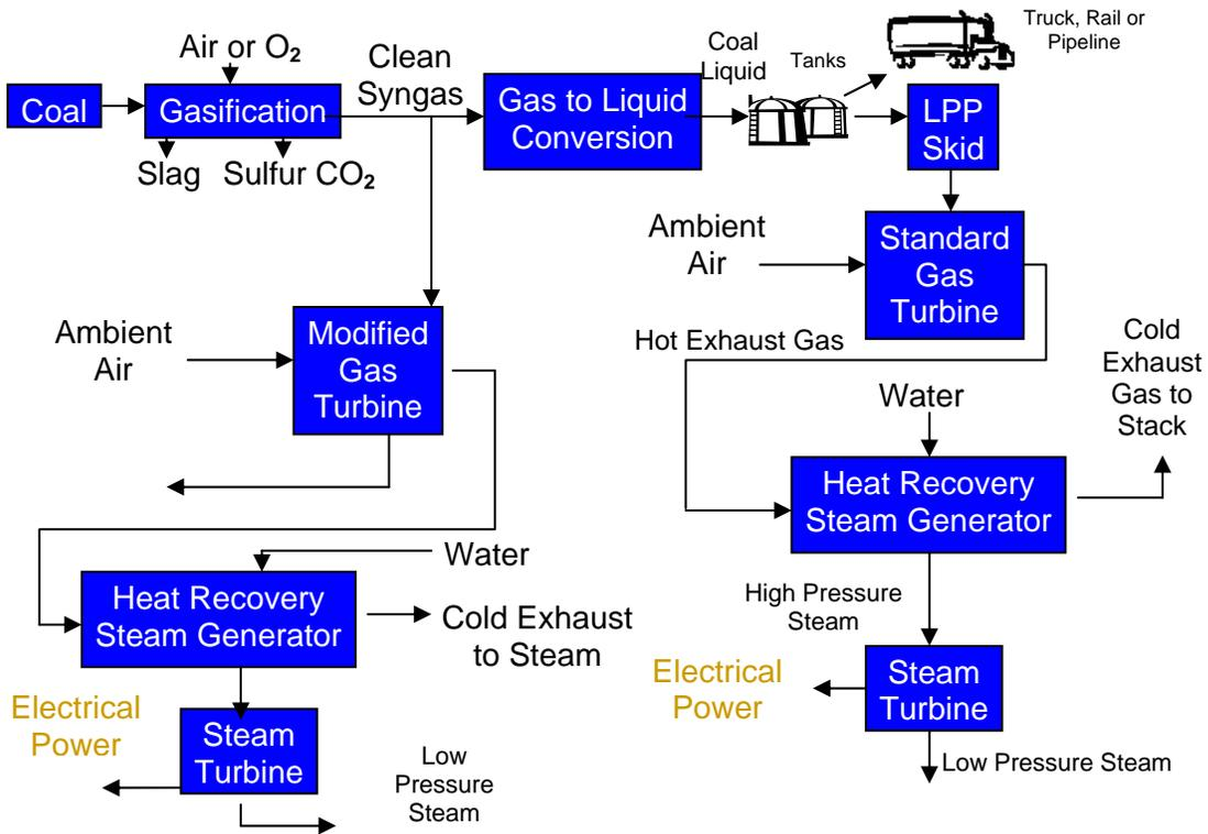
Figure 7: Scenario #2: Integrated LPP Gas™/Syngas IGCC Plant
