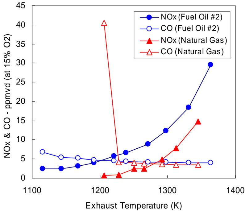
Figure 3: Comparison of NOx & CO emissions measurements for fuel oil #2 and natural gas as a function of measured exhaust gas temperature for a single fuel nozzle at Solar Turbines Taurus 60 full load conditions (100%). Combustion air temperature was 648 K, combustor pressure was 12.6 atm, and fuel dilution was 5:1 (molar basis).
