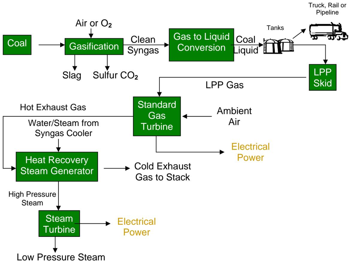
Figure 6: Scenario #1: Integrated LPP Gas™ IGCC Plant
