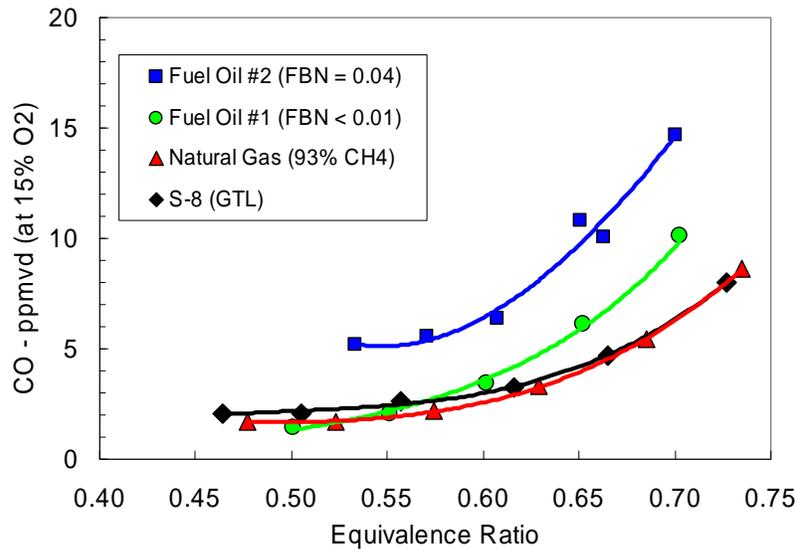
Figure 5: Comparison of CO emissions measurements for fuel oil #2, fuel oil #1, synthetic JP-8 (S-8) and natural gas as a function of measured exhaust gas temperature for a single fuel nozzle at Centaur 50 full load conditions (100%). Combustion air temperature was 627 K, combustor pressure was 1 atm, and fuel dilution was 5:1 (molar basis).
