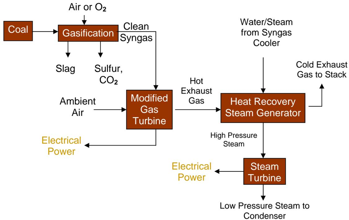
Figure 1: Simplified Typical Coal-based IGCC Plant Process Flow Diagram
