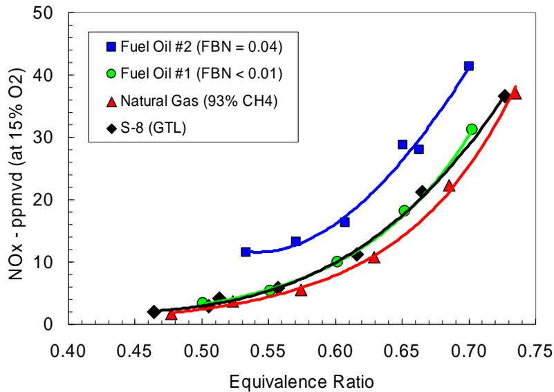
Figure 4: Comparison of NOx emissions measurements for fuel oil #2, fuel oil #1, synthetic JP-8 (S-8) and natural gas as a function of equivalence ratio for a single fuel nozzle at Centaur 50 full load conditions (100%). Combustion air temperature was 627 K, combustor pressure was 1 atm, and fuel dilution was 5:1 (molar basis).
