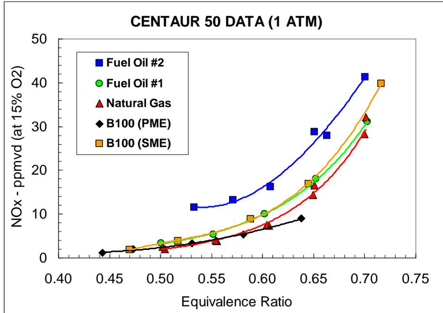
Figure 8. NOx emissions measurements for fuel oil #2, fuel oil #1, natural gas and biodiesel as a function of measured equivalence ratio for a single fuel nozzle at Centaur 50 full load conditions (100%). Combustion air temperature was 625 K, combustor pressure was 1 atm and fuel dilution was 5:1 (molar basis).
