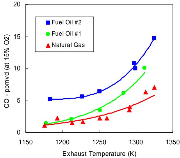
Figure 4: Comparison of CO emissions measurements for fuel oil #2, fuel oil #1, and natural gas as a function of measured exhaust gas temperature for a single fuel nozzle at Centaur 50 full load conditions (100%). Combustion air temperature was 613 K, combustor pressure was 1 atm, and fuel dilution was 6:1 (molar basis).
