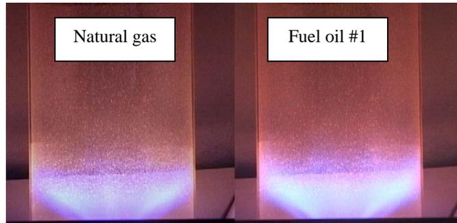
Figure 2: Comparison of natural gas and fuel oil #1 flames at atmospheric pressure for Centaur 50 fuel nozzle at full load conditions.
