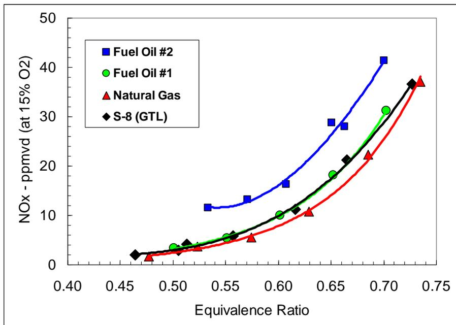
Figure 10: Comparison of  $\text{NO}_x$  emissions measurements for fuel oil #2, fuel oil #1, synthetic JP-8 (S-8) and natural gas as a function of equivalence ratio for a single fuel nozzle at Centaur 50 full load conditions (100%). Combustion air temperature was 627 K, combustor pressure was 1 atm, and fuel dilution was 5:1 (molar basis).
