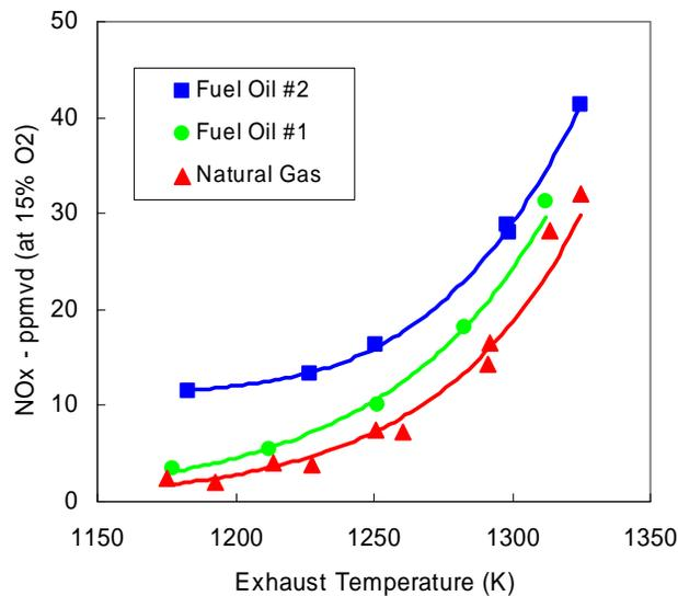
Figure 3: Comparison of  $\text{NO}_x$  emissions measurements for fuel oil #2, fuel oil #1, and natural gas as a function of measured exhaust gas temperature for a single fuel nozzle at Centaur 50 full load conditions (100%). Combustion air temperature was 613 K, combustor pressure was 1 atm, and fuel dilution was 6:1 (molar basis).
