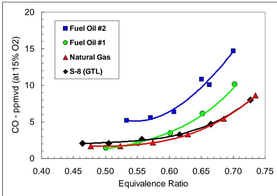
Figure 11: Comparison of CO emissions measurements for fuel oil #2, fuel oil #1, synthetic JP-8 (S-8) and natural gas as a function of measured exhaust gas temperature for a single fuel nozzle at Centaur 50 full load conditions (100%). Combustion air temperature was 627 K, combustor pressure was 1 atm, and fuel dilution was 5:1 (molar basis).
