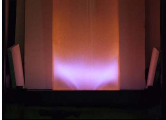
Figure 7: Soy-based biodiesel flame at atmospheric pressure for Centaur 50 fuel nozzle at full load conditions.
