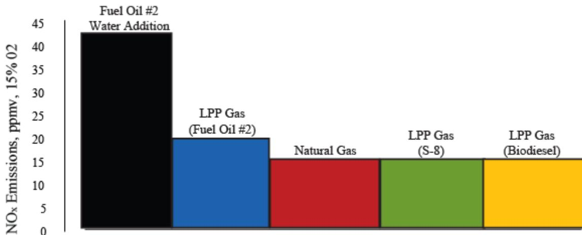
Figure 12: Comparison of NO<sub>x</sub> emission benchmark (42 ppmv) for liquid fuel oil #2 with NO<sub>x</sub> emission performance for fuel oil #2, biodiesel, synthetic JP-8 (S-8) and natural gas for a single fuel nozzle at Centaur 50 full load operating conditions (100%).
