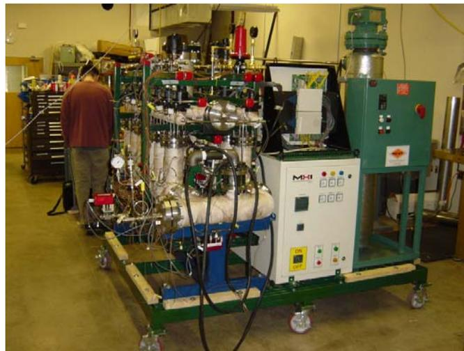
Figure 1: LPP liquid fuel vaporizer skid used for gas turbine burner testing at elevated pressures.
