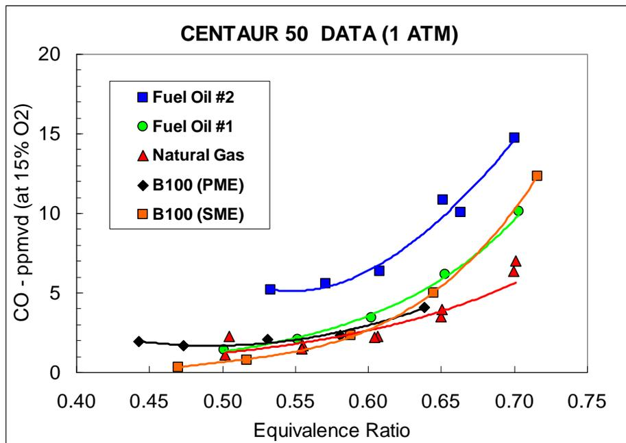
Figure 9. CO emissions measurements for fuel oil #2, fuel oil #1, natural gas and biodiesel as a function of measured equivalence ratio for a single fuel nozzle at Centaur 50 full load conditions (100%). Combustion air temperature was 625 K, combustor pressure was 1 atm and fuel dilution was 5:1 (molar basis).
