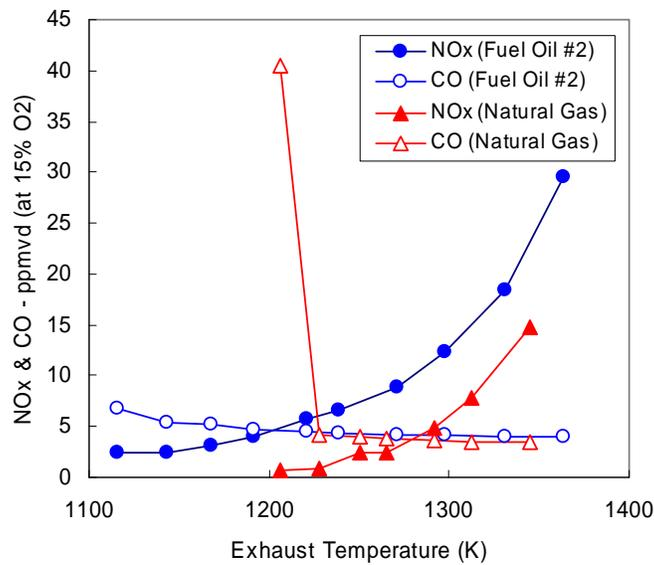
Figure 5: Comparison of NO<sub>x</sub> & CO emissions measurements for fuel oil #2 and natural gas as a function of measured exhaust gas temperature for a single fuel nozzle at Taurus 60 full load
