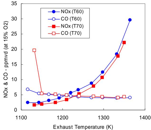
Figure 6: Comparison of NO<sub>x</sub> & CO emissions measurements for fuel oil #2 as a function of measured exhaust gas temperature for a single fuel nozzle at Taurus 60 (T60) and Taurus 70 (T70) full load conditions (100%). Combustion air temperatures were 648 K (T60) and 706 K (T70), combustor pressures were 12.6 atm (T60) and 16.2 atm (T70), and fuel dilution was 5:1 (molar basis).
