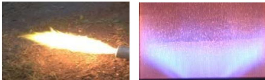
Figure 3: Conventional liquid fuel spray diffusion flame (left) and typical lean, premixed natural gas flame (right)
