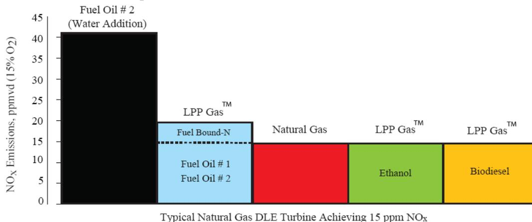
Figure 9: Summary of NO<sub>x</sub> emissions performance for a range of fuels using LPP Combustion technology compared to a nominal 15 ppmv NO<sub>x</sub> natural gas DLE fuel nozzle and conventional spray diffusion nozzle with water addition.
