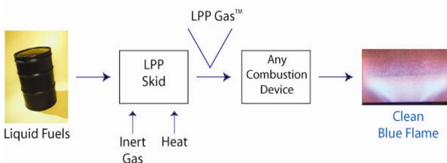
Figure 4: LPP Combustion process diagram
