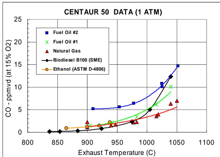
Figure 8: Comparison of CO emissions for natural gas, fuel oil No. 2, fuel oil No. 1, biodiesel (soy methyl ester, SME, ASTM D6751) and ethanol (ASTM D-4806).
