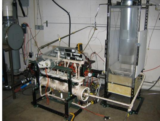
Figure 5: Atmospheric pressure combustor test facility used to evaluate emissions for various fuels using LPP Combustion Technology.
