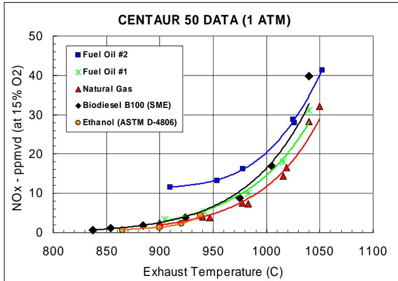
Figure 7: Comparison of  $\text{NO}_x$  emissions for natural gas, fuel oil No. 2, fuel oil No. 1, biodiesel (soy methyl ester, SME, ASTM D6751) and ethanol (ASTM D-4806).
