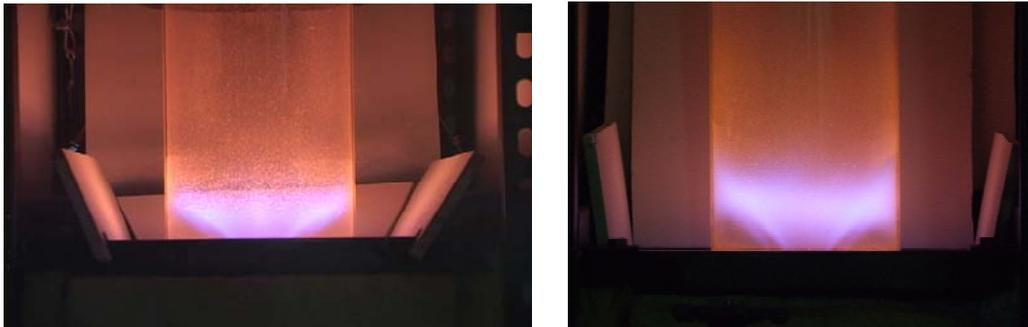
Figure 6: Lean, premixed natural gas flame (left) and lean, premixed, prevaporized biodiesel flame (right)
