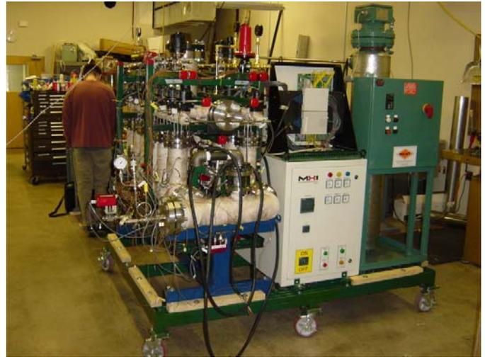
Figure 10: LPP liquid fuel vaporizer skid used for gas turbine burner testing at elevated pressures.
