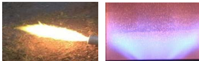
Figure 1: Conventional liquid fuel spray diffusion flame (left) and typical lean, premixed natural gas flame (right).
